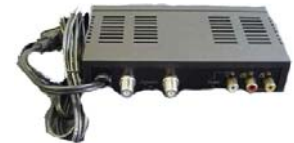
Example of an RF modulator. The DVD player had 2 sets of RCA outputs, one set was connected to the inputs of the modulator unit.
